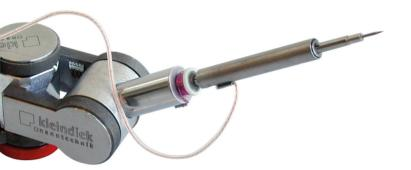
Standard tungsten probe tips can be inserted into the front of the axis and rotated with a resolution of 0.1° per step, allowing applications like true FIB lathe milling, tomography and STEM to be performed with ease. In addition the MGS2-EM microgripper can be combined with the rotational tip to allow gripped objects to be rotated.
