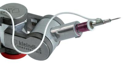
Standard tungsten probe tips can be inserted into the LCMK-EM tip holder. Triax cabling and feedthroughs carry the electrical signals to an adapter which fits all conventional parameter analyzers.
