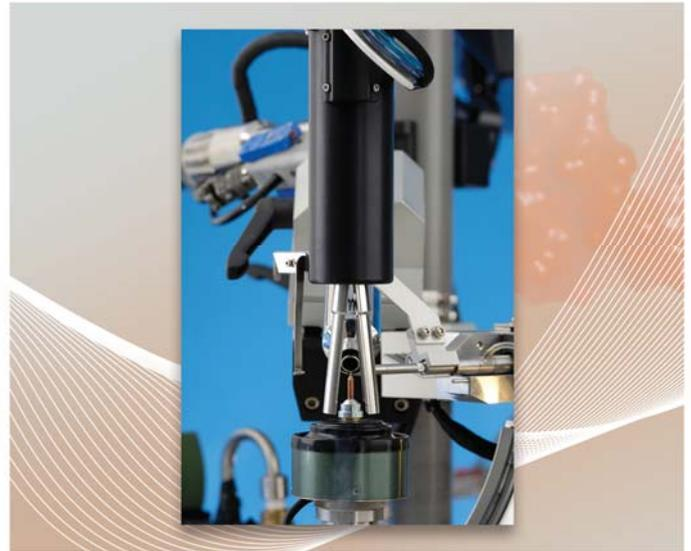
The cryo-resistant ACTOR end effector is designed to eliminate turbulence during sample mounting and dismounting
