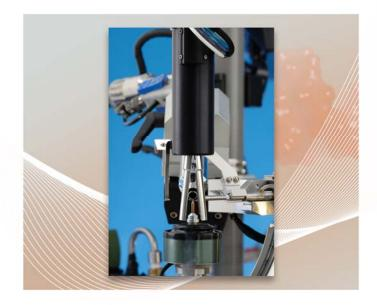
The cryo-resistant ACTOR end effector is designed to eliminate turbulence during sample mounting and dismounting
