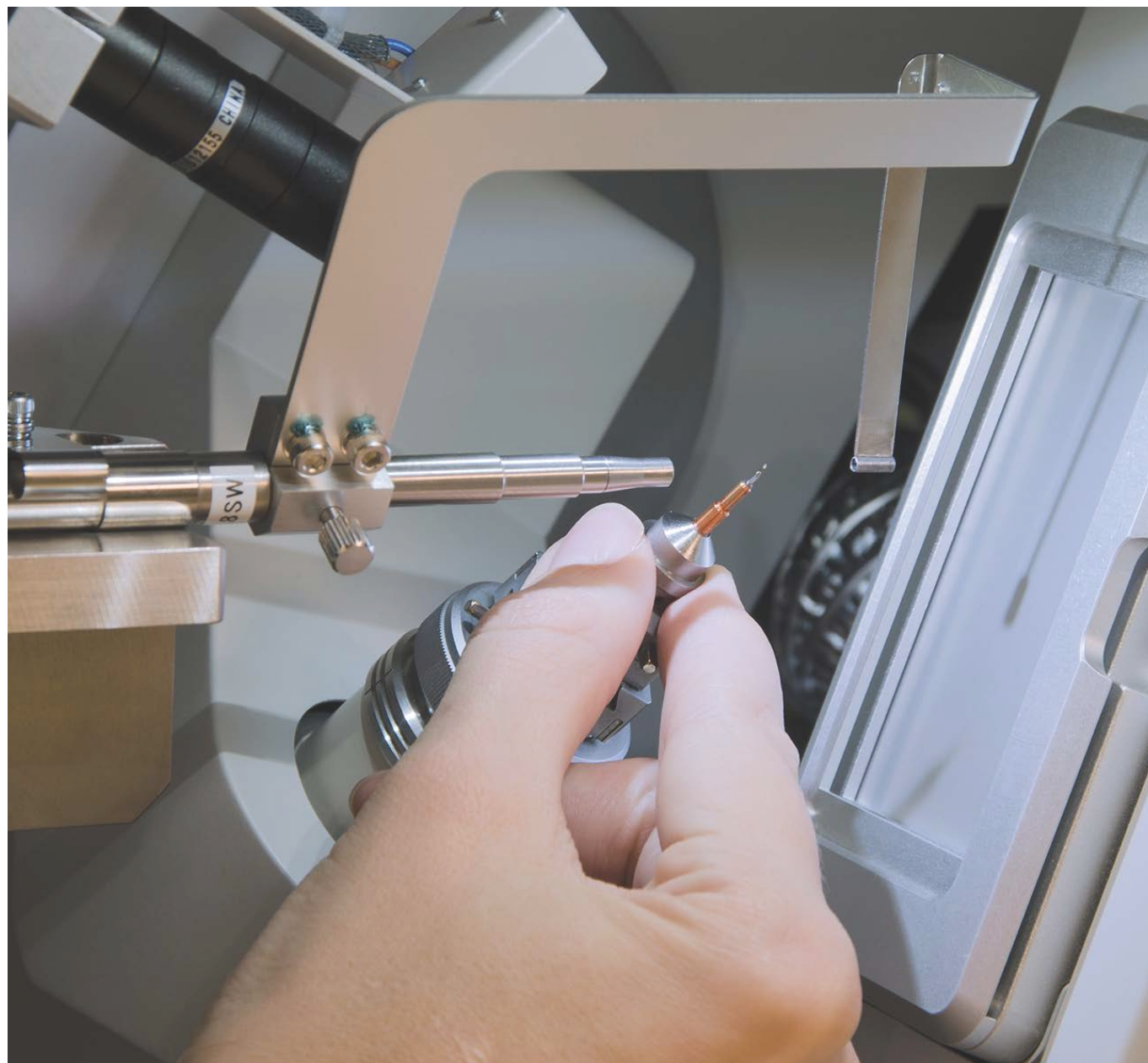
Mounting the crystal on the goniometer head.
