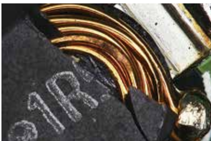
Crack of mounted component (60x, 0 degree)
