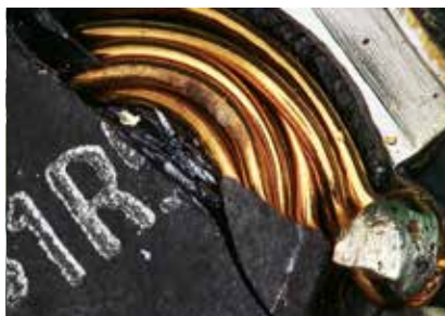
Crack of mounted component (60x, 20 degree)
