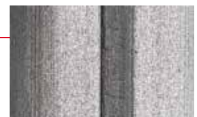
Junction on the inner wall of aluminum pipe (50x)
