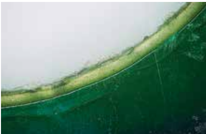
Scratches on circuit board (80x)
