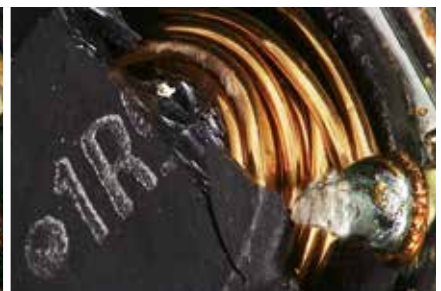
Crack of mounted component (60x, 45 degree)
