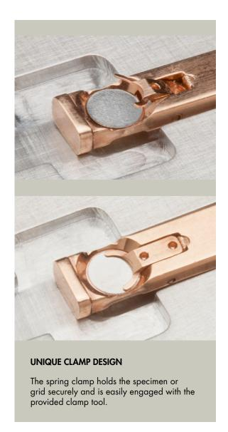
force on the edge of the specimen and maximizes specimen visibility, even at high-tilt angles.
