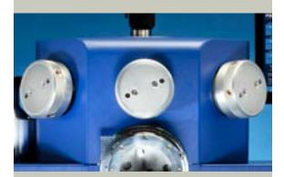
Our patented TrueFocus ion sources are optimized to perform at near 100% ionization efficiency – the result is a highly efficient ion source that maintains a consistent beam current. This technology is built into the Model 1062 TrionMill.
