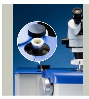
A thermal safeguard can be programmed to a specific stage temperature threshold at which the ion sources will be deactivated if the liquid nitrogen in the dewar becomes depleted.
