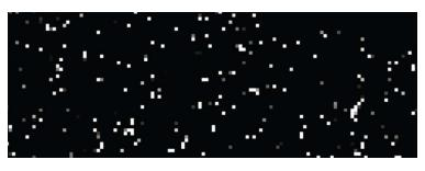
The DE-64 delivers ultra-high DQE(0) because electron events are easily distinguishable from background. The counting threshold is thus highly effective.
