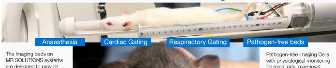
are designed to provide important support functions to the animal during the preparation stage and throughout the imaging process. The beds provide anaesthetic gas to the animal and thermo-regulation of the animal during the scan.
