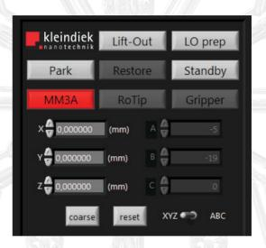
By 'talking' to the microscope, the software is able to adjust the micro-manipulator's speed of motion to match the given magnification. The software also provides true Cartesian motion using the microscope PC's mouse (for X and Y motion) as well as an additional USB jog shuttle device (for Z motion). In addition, the software is equipped with park&restore functionality and can be used to control the microgripper.
