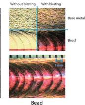
On the weld bead, the residual stress is approximately equal to zero. Tensile stresses from 200 MPa to 300 MPa are observed in the heat-treated area in the base metal. In the sandblasted area, the mapping chart shows that the tensile stress has changed to the compressive stress of about -1000 MPa by the sandblast treatment. By using the CCD camera with a zoom function, the images of the sandblasted and non-sandblasted areas are recorded as shown in the left pictures.
