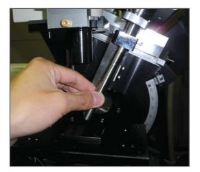
Residual stress in a micro area is measured by utilizing optional collimators. The collimators are easy to install and remove. Optional sizes are:  $\varphi$ 30 µm,  $\varphi$ 50 µm,  $\varphi$ 100 µm, as well as  $\varphi$ 300 µm,  $\varphi$ 500 µm,  $\varphi$ 2 mm, and  $\varphi$ 4 mm. Standard collimator sizes are  $\varphi$ 150 µm and  $\varphi$ 1 mm.
