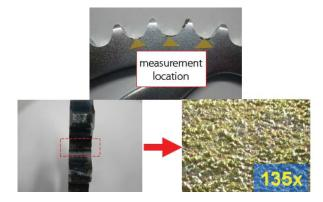
A CCD camera equipped with a microscope with a zoom function is used to select the measurement position (Magnification : 22x to 135x). By using the computer controlled XYZ sample stage, a measurement position can be selected remotely and the image of the measurement position can be recorded. The image to the left shows the bottom of a gear between two teeth.
