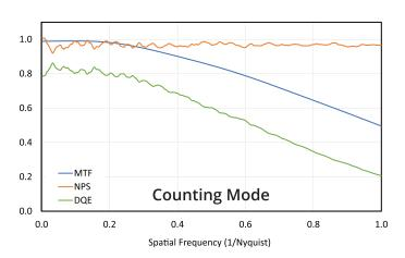
DQE curves are shown for 300 kV electrons | Specifications and performance are subject to change. Example images of various camera applications were collected by researchers using one of Direct Electron's cameras (not necessarily the DE-16)
