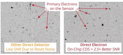
Direct Electron's DDD® sensors have ultra-low noise, which is clearly demonstrated by visualizing individual 300 keV electrons. TEM primary electrons clearly stand-out from the background on the Direct Electron sensor, while they are often lost in the background of other sensors. Figure courtesy of Greg McMullan, (MRC-LMB, Cambridge, UK).
