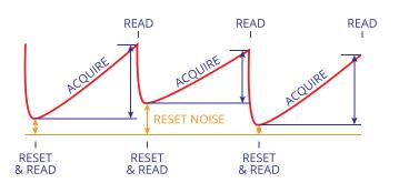
on-chip correlated double sampling (CDS) dramatically improves sensitivity by subtracting reset noise that plagues other CMOS sensors
