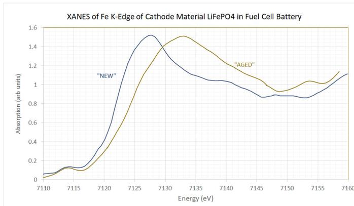
**Figure 2:** XANES spectra of  $\text{LiFePO}_4$  cathodes at different charge/discharge states. QuantumLeap-210 scaled acquisition time and energy resolution for each cathode sample are 3 hours @  $\sim 0.5$  eV.
