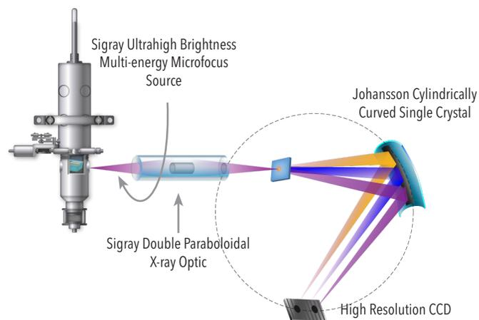
**Figure 1:** QuantumLeap's XANES off-Rowland geometry: Sample is placed within the Rowland circle to enable simultaneous detection of multiple wavelengths (vs. conventional energy scanning approach, which is lower throughput). High energy resolution of <0.5 eV is achieved by using Johanson crystals coupled with a high resolution CCD.
