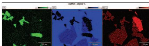
Figure 6: O, S and Mo in a composition image separated by atomic percentage using Quantitative X-ray Mapping
