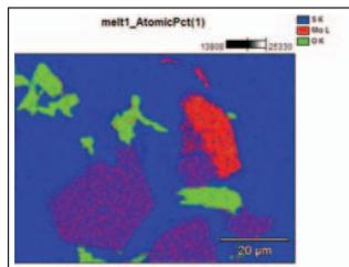
Figure 7: Sulfur and molybdenum spatially separated
