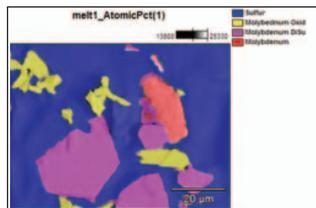
Figure 9: Composite distribution of the four sulfur and molybdenum phases above
